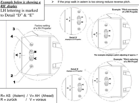
independently for forward and reverse. The turning of the adjusting screws (2) & (4) in Figure "Example" by half a revolution changes the pitch approx. 1". That means a quarter turn (90°) changes the pitch by ½" and a one full turn by 2" etc. For a check of pitch adjustments there are markings on the hub rotating flange. To return to original factory pitch settings, line up "V" resp. "R" markings on the hub face. (see example beside)
