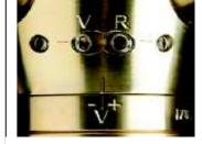
Marked lettering of a LH Propeller
