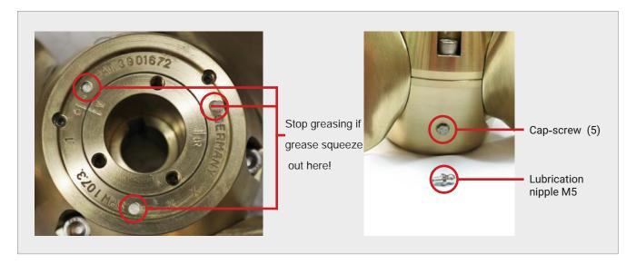
Factory supplied special grease EP/SAL is recommended and available from your VARIPROP distributor. Avoid regular white grease (sterntube-grease)!
