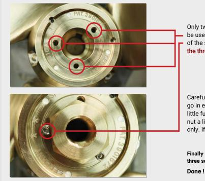
Only two of the three lock-pin holes can be used, depending on the final position of the shaft-nut flange. At least one of the three tapped holes must be used.
