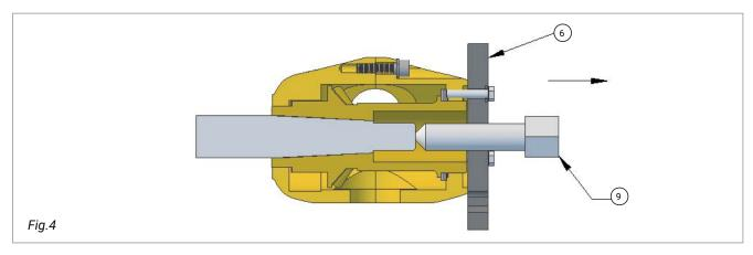
4. Now turn the hexagonal head bolt (9) against the end of shaft until the VARIPROP comes off the taper. Do not use excessive force to turn bolt (9). If prop does not come off, proceed to page 10 -> removal after the 3rd season. Never use a hammer to remove the prop from the taper !!!
