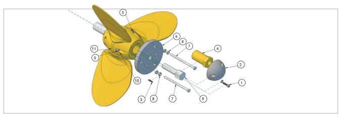
3. Then remove at first only two hexagonal socket screws (5). DO NOT OPEN ALL!!
