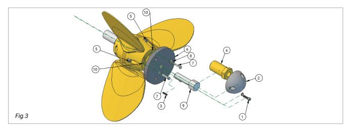
3.) Fit the short hexagonal head screws (7) into the inner bolt circle diameter of the puller (6). Fit the SPW puller (6) onto the aft of the rear boss and screw the short hexagonal head screws (7) completely into the zinc screw holes (10). Take care that plate (6) will fit snugly and evenly to the aft boss.
